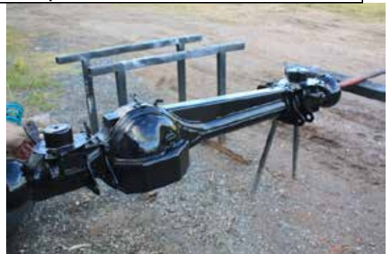
Figure 1: Weld On Diff Brace Fitted To The Diff.
