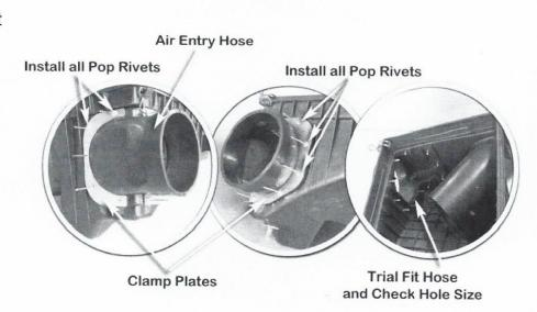
With all of the pop rivets installed, place a body washer (item 17) onto each pop rivet, secure the pop rivets with a pop rivet gun starting from the corner of the air cleaner housing and working outwards.
