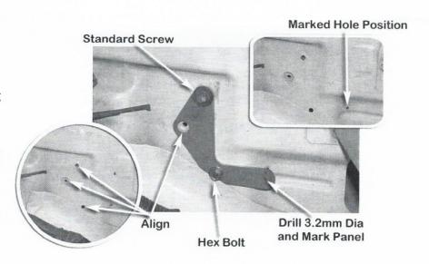
Use a centre punch to punch the centre of the hole accurately, this will ensure the drill stays central whilst drilling.
