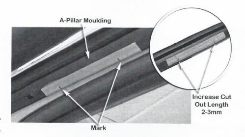
Use a body saw to remove the marked section of the Apillar moulding, cutting through the channel and into the right angled section by approximately 2 – 3mm as shown, use a file to neaten all of the cuts.
