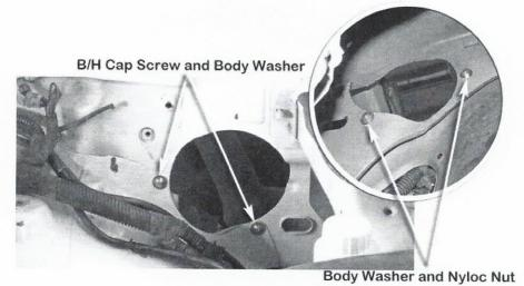
Align the filler neck template (item 30) to the standard holes in the inner guard panel shown.
