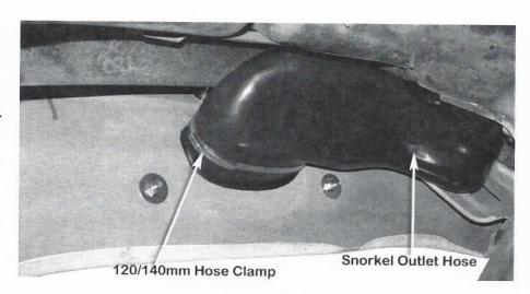
Install the air cleaner element, air cleaner housing top, side indicator, guard liner and any other components removed during the installation process, top up the washer bottle with washer fluid, install the filler neck cap (item 24) and check washer operation.
